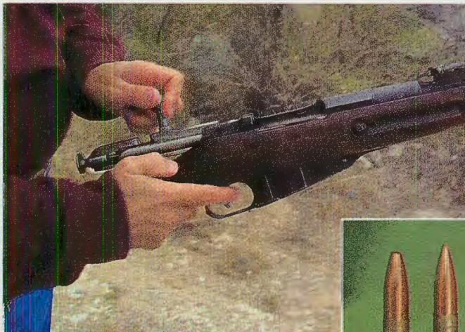
The Mosin bolt is readily removed for cleaning by retracting to the rear, pulling the trigger, and withdrawing it. (inset) Typical reloads include author's homemade 174-grain JHP built on a Corbin swaging setup, Sierra 174-grain match bullet, Hornady 180-grain round nose, and Hornady 123-grain soft point.
